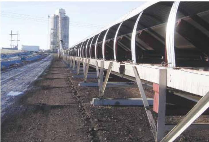
*In conjunction with Roberts and Schaefer, AC-Tek designed and commissioned this 3,3 km long, 7 000 t/h conveyor (with an 1 830 mm belt) at the huge Black Thunder coal mine in Wyoming in the US. Owned by Arch Coal, Inc, Black Thunder produces nearly 3 tons of coal per second around the clock, sufficient to fill 18 to 20 trains a day. It is one of the largest coal mines in the world accounting for nearly 9 % of US production.*
