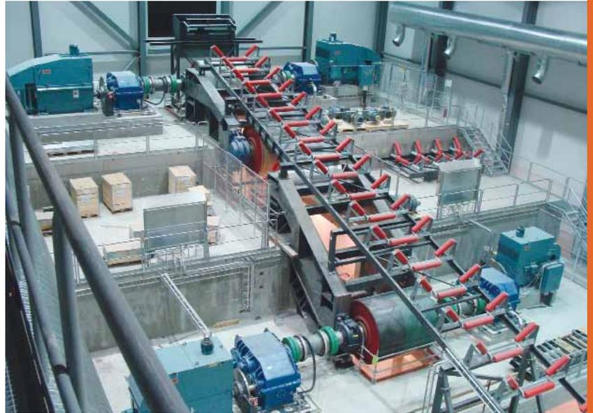
*Current construction progress at the 9 200 kW head drive station for the 8 000 t/h incline conveyor at Aitik, Sweden. According to David Kruse, the design contains significant advancements in conveyor technology and is one of the largest belt conveyor systems currently under construction.*
