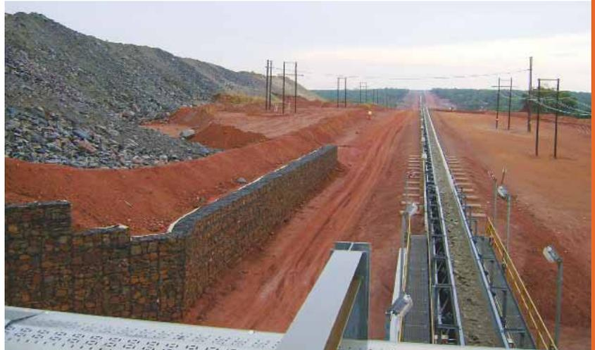
*The 4,3 km long overland conveyor at Equinox Minerals' Lumwana copper mine in north-west Zambia. The contractor was SMH with AC-Tek providing specialist input. Lumwana is probably the biggest copper mine in Africa.*
